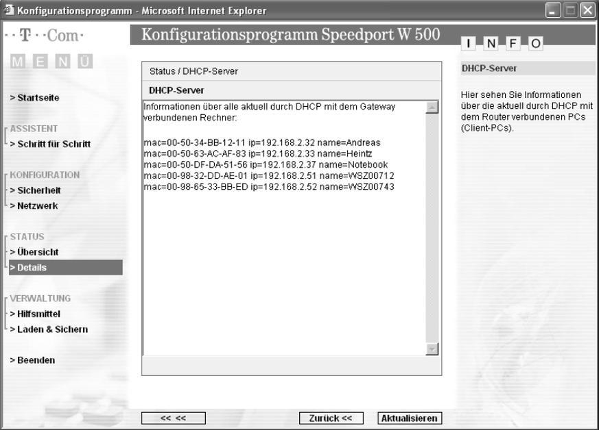
The screenshot shows the 'Konfigurationsprogramm Speedport W 500' interface. The main window displays the 'DHCP-Server' status, listing information for all currently connected DHCP clients. The interface includes a navigation menu on the left and a status bar at the bottom.
